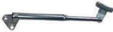
FIRMOTOP STAY 000345 130mm, chrome finish cupboard stay-up. Spring pressure supports the flap when raised and holds it firmly against the cabinet when closed. One or two stays are required depending on weight of flap.
